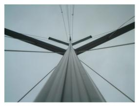
Your sailing rig is a safety critical system which must be in good order and well tuned, neglect it at your peril. Insurers usually require the standing rigging to be replaced every 10-12 years for pleasure use, with the interval reducing rapidly for serious sailing, racing or charter. Ask when the standing rigging was last renewed and if there has been a recent aloft rig and spar check.
